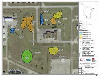
During soil excavation, an X-ray fluorescence (XRF) analyzer will be used in the field to determine lead concentrations. Soil above the NTCRA criteria for lead in residential soils (i.e., 358 milligrams per kilogram [mg/kg]) will be excavated and disposed off-site. If XRF results
